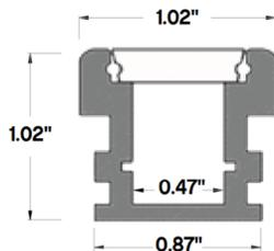
A durable in-ground aluminum channel designed for pavement, sidewalk, and driveway applications. Included polycarbonate frosted diffuser is certified for all weather conditions, UV resistant, and can withstand a maximum load of 5000 lbs.
