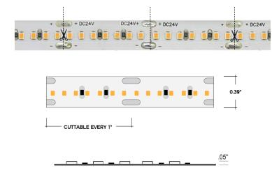
TBD.S81 is a high-output linear lighting system designed to provide a continuous light source without hot spots. At 5.5W per foot, produces over 500 lumens per foot! Low profile, for use with shallow profile channels. Superior choice for wall washes and vanities, for indoor use on residential / commercial projects. Fully dimmable, 120 degree beam spread.
