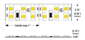
TBD.DS72 is a linear lighting system optimal for areas where high-intensity levels of light are desired. Great for many indoor, commercial / residential applications. With several LED color options and 120° beam spread, this LED strip is a superior option for general lighting: coves, slots, or vanity mirrors. This strip, with high density, double-row LED spacing, when used with a deep channel and frosted lens, virtually eliminates all hot spots.
